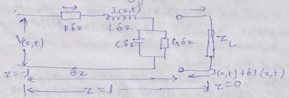
Considering the voltage and the current relations along the line, as shown in figure 0 i.e.  $(\frac{31}{32}) + C(\frac{3V}{3V}) = 0$  and  $\frac{3V}{3Z} + L(\frac{31}{3V}) = 0$
